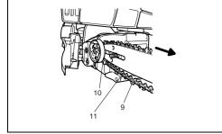
Lift the chain (9) over the sprocket (10). Using your right hand, guide the chain into the top guide groove (11) on the guide bar.
